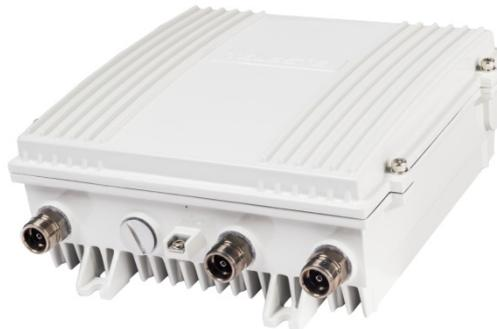
The AC3010 is a single active output amplifier with 48 dB maximum gain. The amplifier stages are based on extreme high performance GaN solution that makes the usable gain range especially wide and allows high output level. Integrated interstage gain and slope controls optimise the flatness performance.
